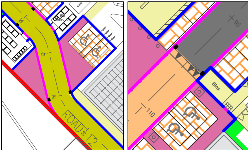
Figure 11 | Examples of Horizontal Deflection (Road Curvature) left, and Vertical Deflection (Ramps) right
